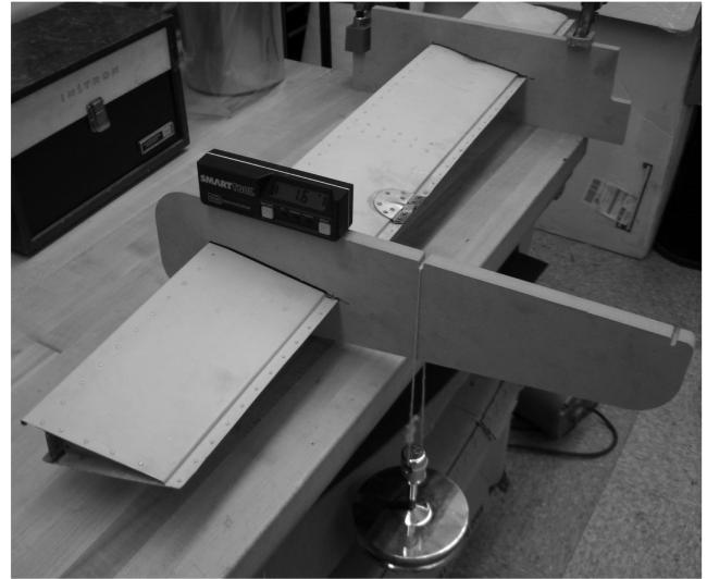
Fig. 9 Torsional test of small control surface with bearing block mounted at trailing edge.
