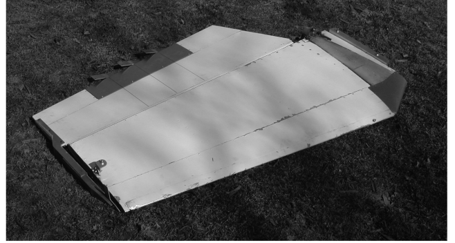
Fig. 6 Modified half of a Cessna 150 horizontal stabilizer, equipped with servo controlled canted tabs.
